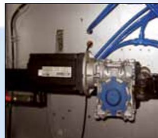
Servo drive with integrated breaking facility for paper pull for precise control of pouch height.
